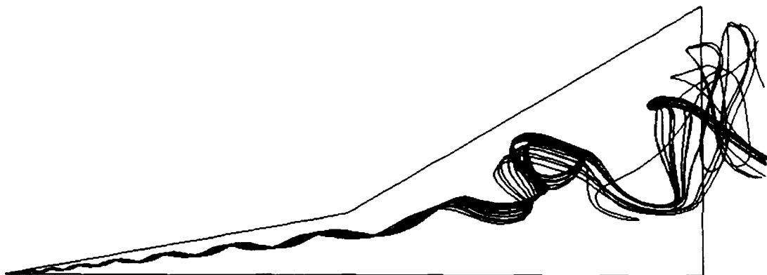
Figure 5. Computed off-surface particle path pattern; M_\infty=0.3 , Re=1.3 \times 10^6 , \alpha=35^\circ
